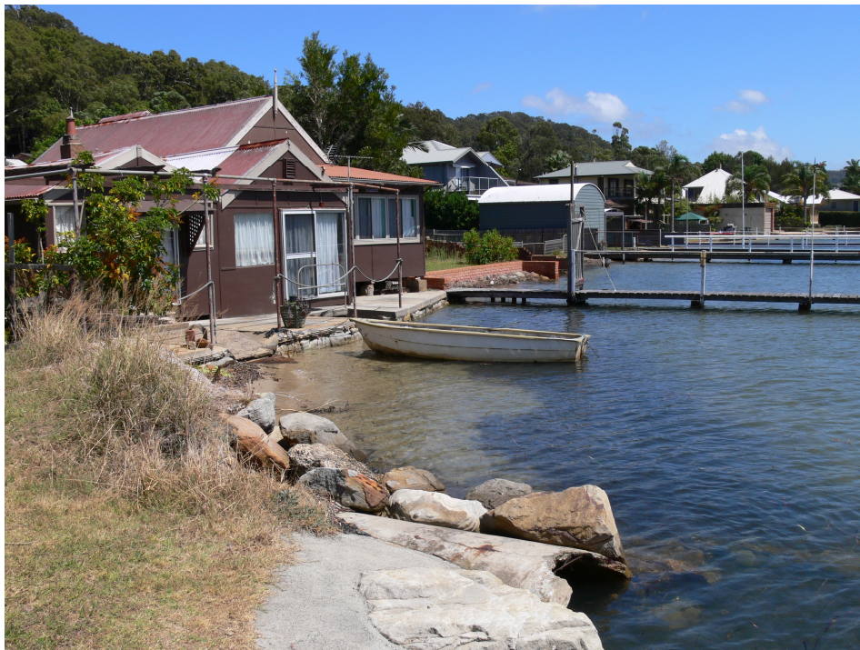
Figure A8. Limited freeboard to floor levels at Pretty Beach, Brisbane Water, Central Coast. Photo: Fiona Lambell.
